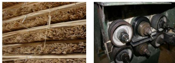
Figure 49: "crushing" des lamelles
